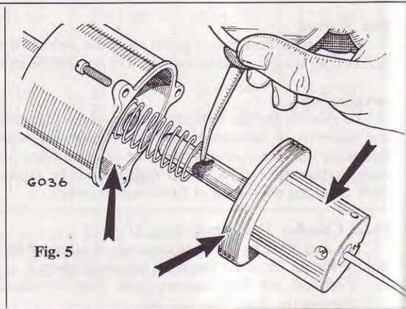
The needle size is engraved on the shoulder of the needle, which should be fitted with the shoulder flush with the under face of the piston and retained by tightening the screw.
