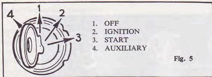
position the key may be withdrawn ; 2, "Ignition" ; 3, Start ; 4, Auxiliary. (See Fig. 5.)
