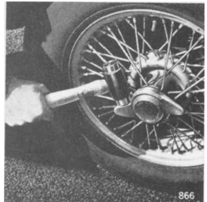
Fig. i8. Removing L.H. front hub cap.
