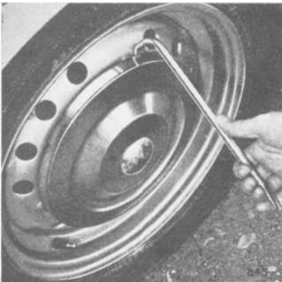
Fig. 17. Removing nave plate.
