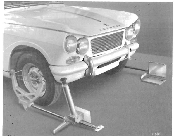
Fig. 2. Using Dunlop optical wheel alignment gauge
