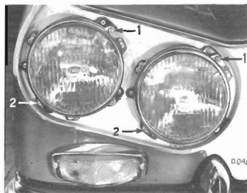
Fig. 55. Beam alignment adjustment screws
