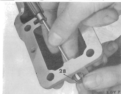
Fig. 11. Removing rubber 'O' ring from extension
