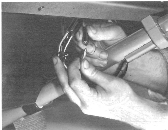
Fig. 30. Reconnecting cables at snap connectors
