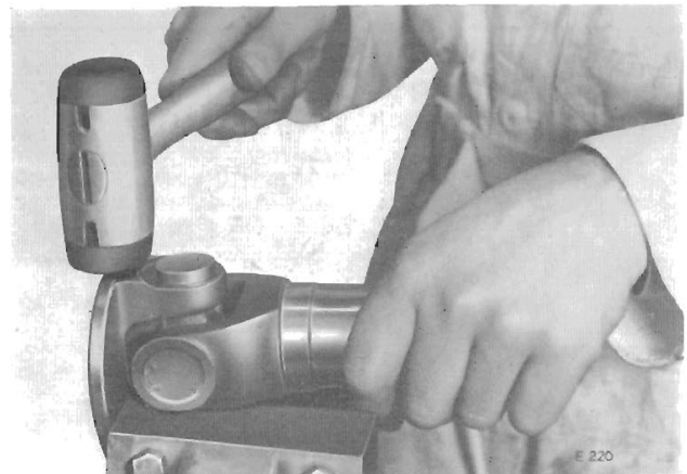
Fig. 6. Removing a bearing cup from the flange
