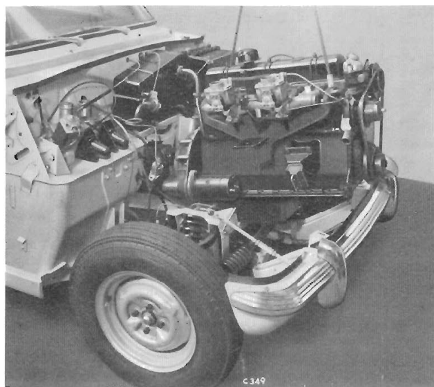
Fig. 13. Using sling to remove engine and gearbox
