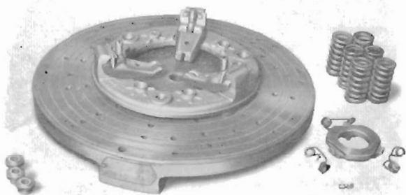
Fig. 20. Assembling toggles to pressure plate (Herald and Spitfire)
