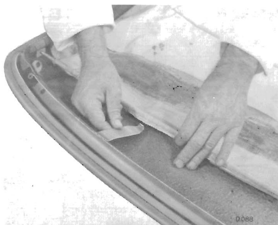
Fig. 30. Assembly No. 1 listing rail to retaining clips
