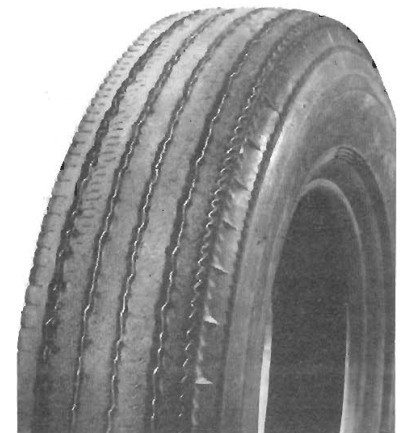
Fig. 9. Tyre wear resulting from front wheel misalignment
