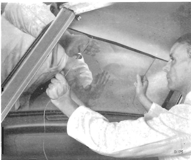
Fig. 67. Pulling the cord to turn the lip of the rubber over the body flange
