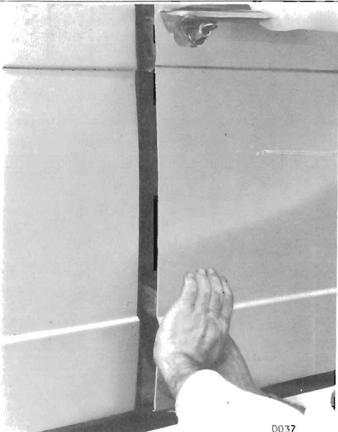
Fig. 43. Inserting wedges to increase gap
