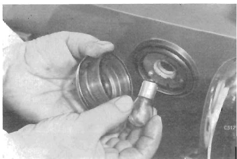
Fig. 59. Front parking and flasher lamps (Spitfire)
