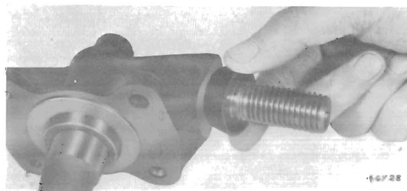
Fig. 16. Fitting rubber seal to vertical link
