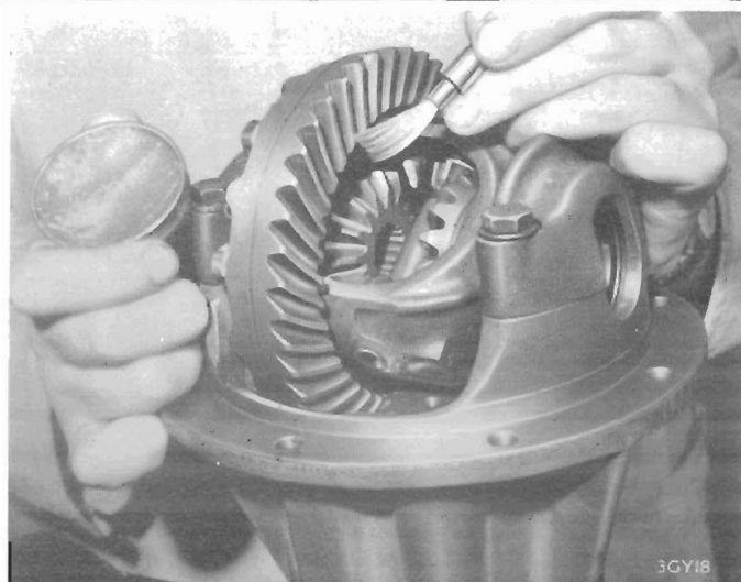
Fig. 51. Painting crown wheel teeth to check pinion marking
