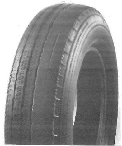
Fig. 7. The results of excessive front wheel camber
