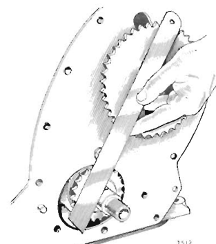
Fig. 67. Checking sprocket alignment
