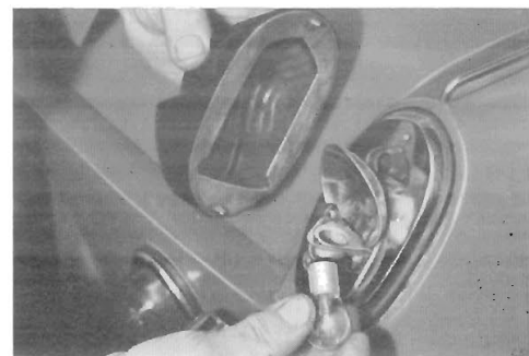
Fig. 61. Tail/stop and flasher lamps (Spitfire)
