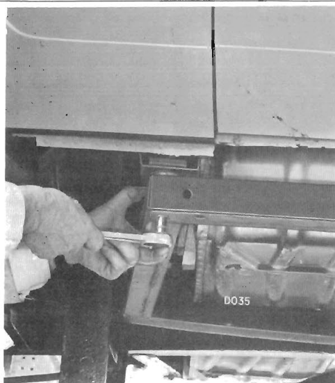
Fig. 42. Re-tightening body bolts
